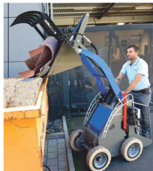
Useful for clearing work with the bucket
